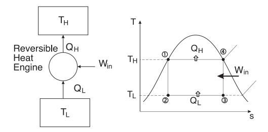
$$egin{array}{lll} W_{in} & = & Q_{net} = Q_H - Q_L \ & = & (T_H - T_L)(s_3 - s_2) \end{array}$$
